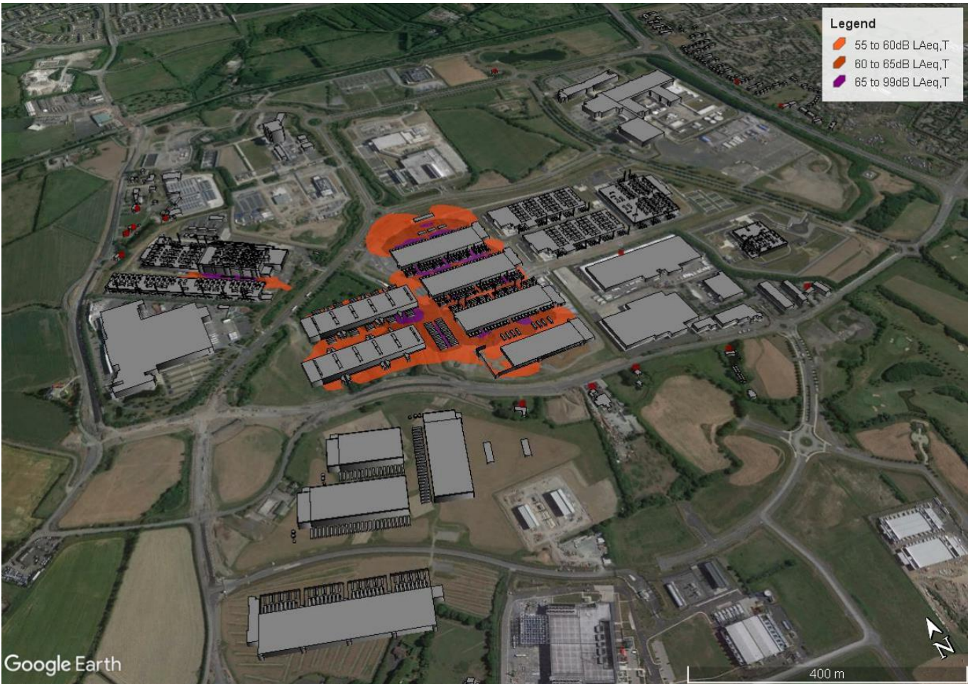
Figure 8.9: Scenario D – Generator Testing (with DUB 14 and 15) Contour (Extent of 55dB(A) Contour
